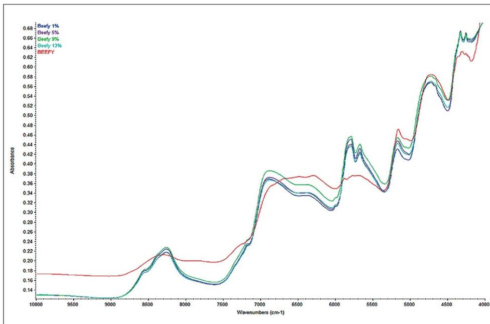
Figure 4: NIR spectra of pure beefy flavor (red) and crisps with 1 to 13% flavoring
