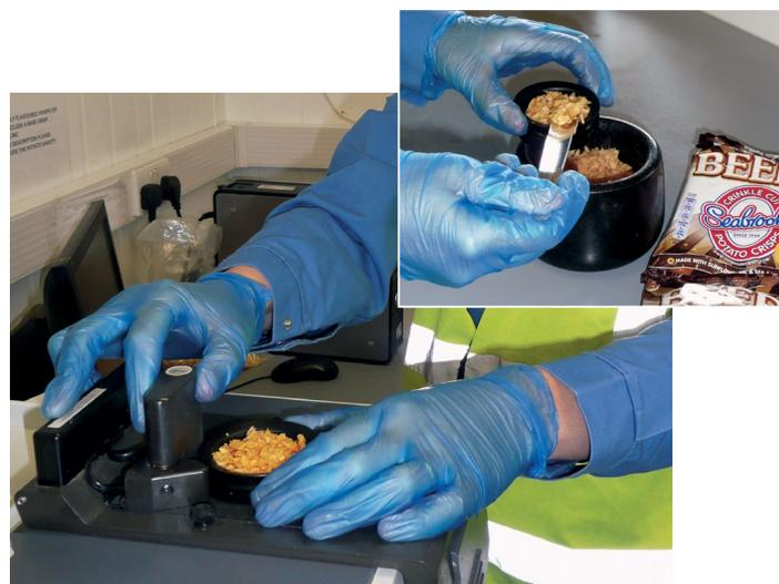
Figure 3: Potato crisps are ground by a mortar and pestle (inset) then loaded into the Sample Cup Spinner accessory of the Antaris II MDS system
