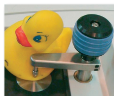
Figure 1: Smart iTR accessory in a Nicolet iS10, showing a sample being analyzed nondestructively
