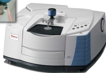
Figure 1: Smart iTR accessory in a Nicolet iS10, showing a sample being analyzed nondestructively
