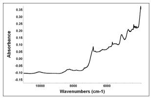
Figure 2: Representative spectrum of an ascorbic acid-starch mixture used as a standard
