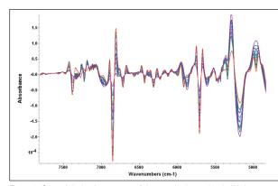
Figure 3: Second derivative spectra of the standards used to build the chemometric model. The variation between the standards is clearly shown in the range from 4800 to 7600 cm<sup>-1</sup>.
