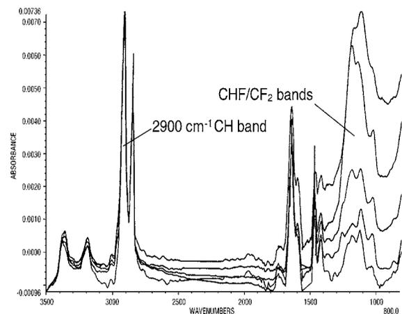
Figure 3: Series of calibration spectra obtained for fluorinated polyethylene samples. Bands used for determination of fluorination levels are indicated.
