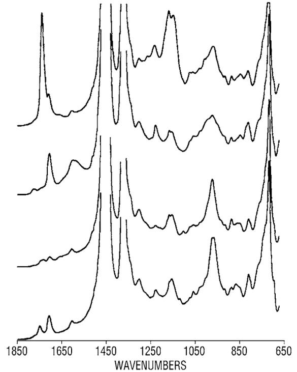
Figure 5: Overlay spectra of commercial lubricating oils showing differences in base oils and additives.
