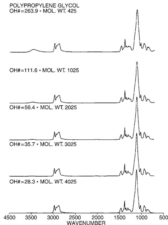
Figure 7: Spectra of polypropylene glycol samples with different hydroxyl values.
