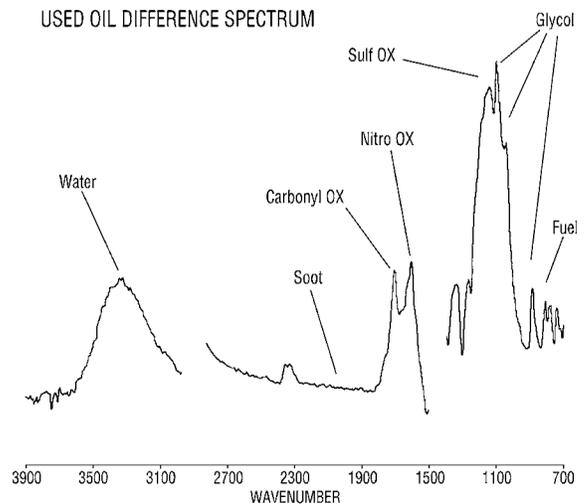
Figure 6: Typical used engine oil difference spectrum with components of interest labeled.
