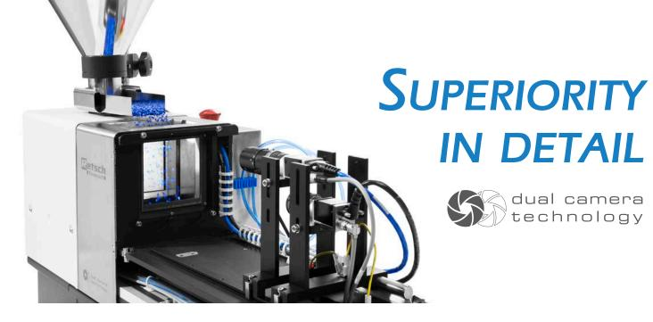
The innovative CAMSIZER P4 measuring system is based on the Dynamic Image Analysis principle. The bulk material falls between light source and cameras. Each particle is detected by the cameras with a high frame rate, and is then digitalized and processed by the connected computer.
