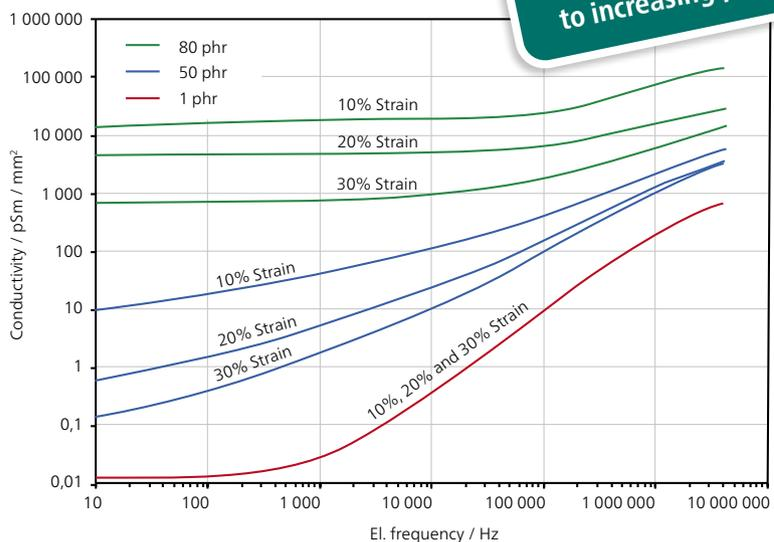
DiPLEXOR® measurements on HNBR with different levels of carbon black N550 content: 80 phr, 50 phr and 1 phr in compression mode at 25°C.
