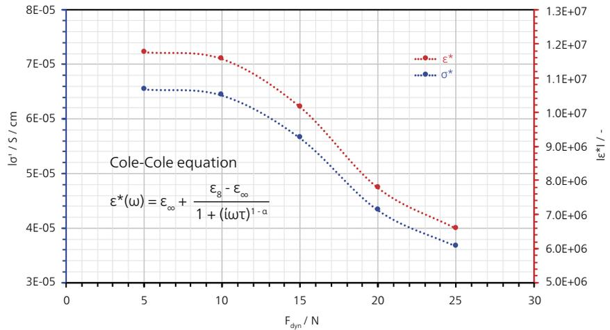
SBR 70 phr\* N 234 at  $F_{stat}$  30 N,  $f$  10 Hz and  $f_{el}$  10 Hz; conductivity and permeability versus dynamic force amplitude varying from 5 N to 25 N in steps of 5 N
