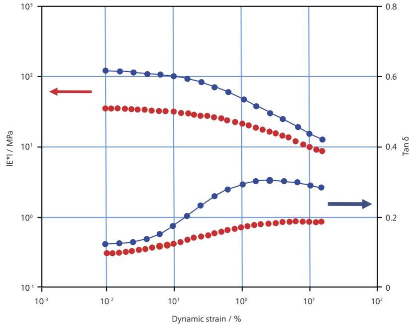
Stiffness and damping of two different elastomeric systems depend on the applied dynamic strain.
