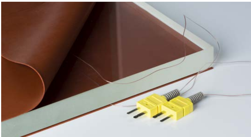
Thermocouples can be placed in the specimen's center
