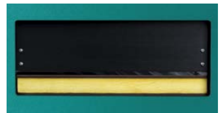
Various plate openings of the NETZSCH HFM 446 Lambda are possible when changing the specimen
