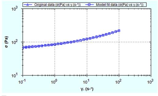
2 Shear stress-shear rate data for the Carbopol-based hair gel with Hershel-Bulkley model fit
