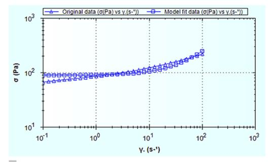
3 Shear stress-shear rate data for the Carbopol-based hair gel with Bingham model fit
