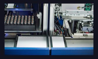
With a capacity of up to 75 vials, the Module APPLICATION is designed for autonomous application of multiple samples on up to five different plates. For this, we recommend the Module PLATE STORAGE, which automatically feeds the Module APPLICATION with new plates. The Module APPLICATION supports the application of more than 200 samples per day.
