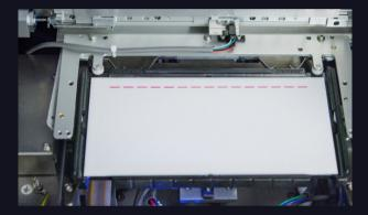
The plate containing the samples is ready to be loaded into the developing chamber.
