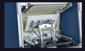
The tilting mechanism lifts the plate from its horizontal position to the vertical position in the developing chamber and the plate is developed according to the method chosen.
