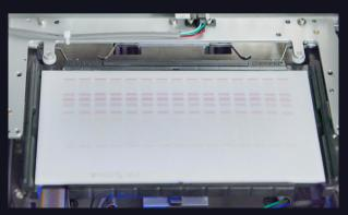
After processing in the developing chamber, the developed plate is brought back into the horizontal position, ready to be moved from the Module DEVELOPMENT to other modules for further processing.
