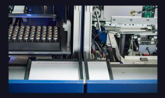
After application of all samples, the plate is moved to the Module DEVELOPMENT.
