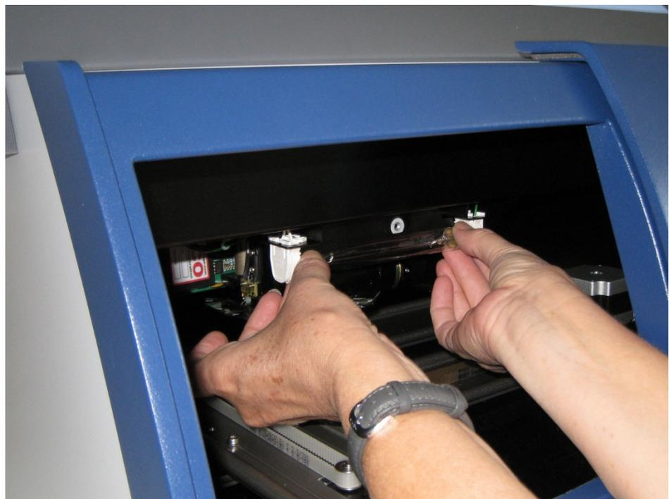
*Fig. 11: Replacing the compartment illumination lamp.*
