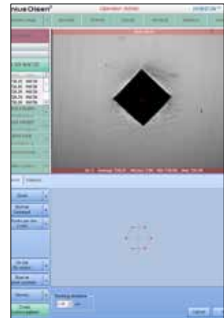
Screen 2: User-defined pattern/sequence of Hardness measurement locations.
