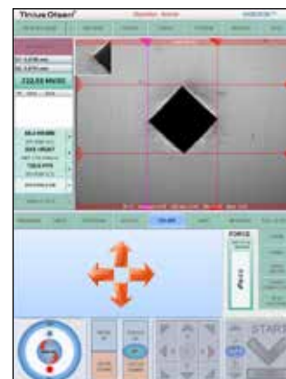
Screen 4: Filar lines option to manually define the precise edges of the indent, along with the zoom measurement option.
