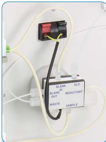
New valve concept to conserve reagents
