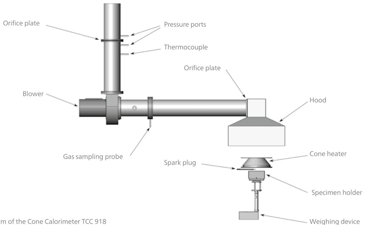
Schematic diagram of the Cone Calorimeter TCC 918
