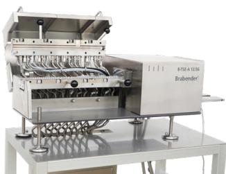
Clam Shell Design - openable liner for optimum process monitoring and easy cleaning
