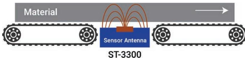
The ST-3300 is an open-frame configuration that is installed between conveying belts or rollers exiting or entering a kiln or dryer. Antenna lengths are available from 15 – 244 cm (6 – 96 in.) dependent upon temperature.
