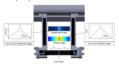
TIMAwave is based on the principle of Ångström's method, a well-known method for the determination of the thermal diffusivity of solid materials. It is a transient method which is based on the damping of one-dimensional thermal waves which are excited using a laser diode to propagate through the sample.
