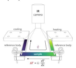
Samples are measured between two metal reference bodies that are known in geometry and physical properties. Measuring both temperature gradient  $\Delta T$  over and heat flow Q through the sample returns its thermal conductivity.
